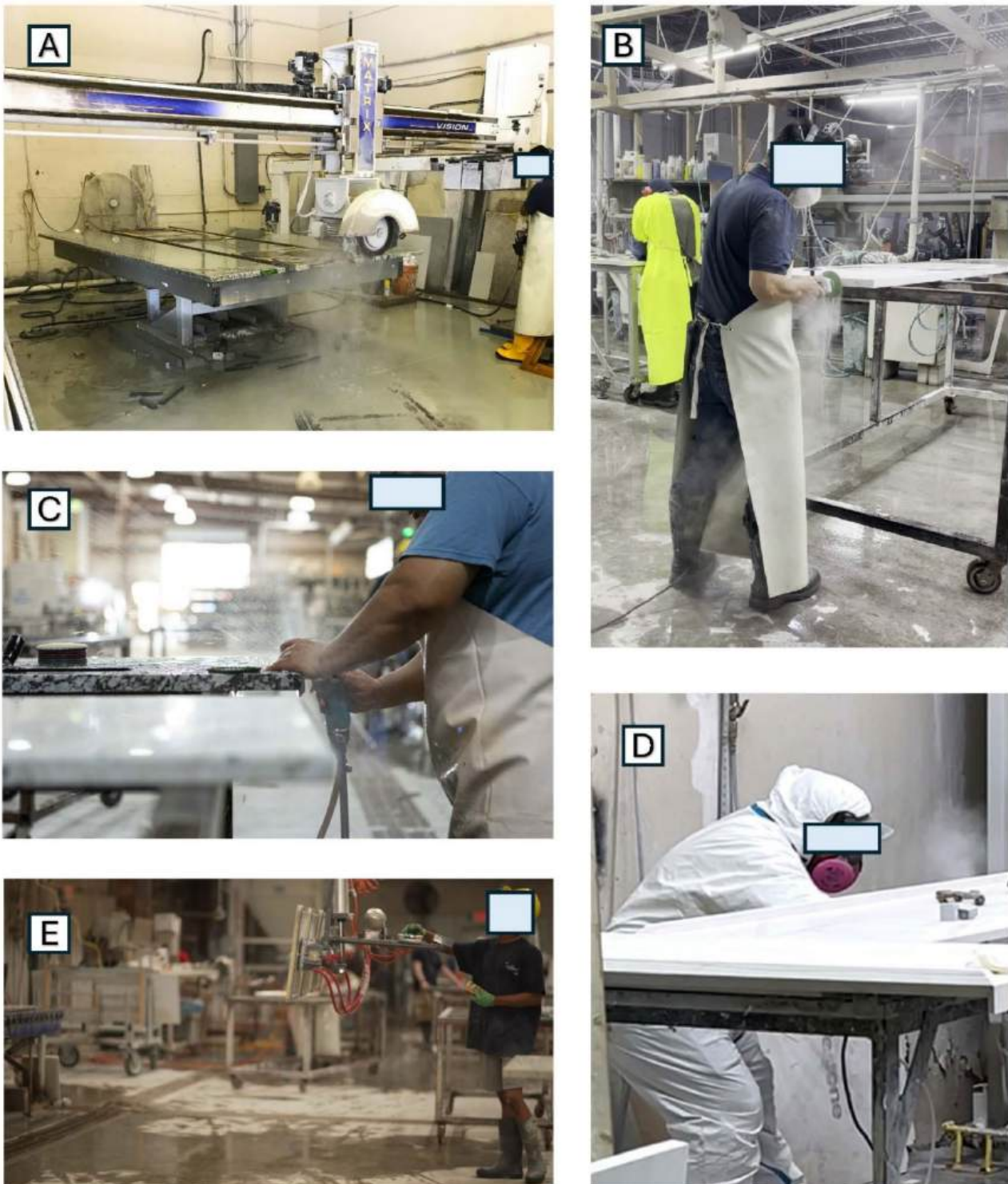
Fig. 3 Examples of jobs and tasks conducted by countertop fabricators. A Automated Tool Operator using a Bridge Saw with Water Delivery. B An employee using dry polishing on an ES slab generating respirable crystalline silica. C Employee wet polishing. D Fabrication of edge following lamination of countertop edge. E Support employee positioning the hoist to lift a slab. Picture Credit: A, B, and D by Jenny Houlroyd, Picture C and E by Mixed Bag Media
